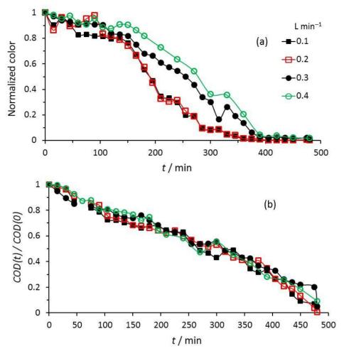
**Figure 5.** Normalized color ( $\lambda$  = 639 nm) **(a)** and COD **(b)** decay during the electrolyses of indigo on ( $Ti/IrO_2$ - $SnO_2$ - $Sb_2O_5$ ) in the FM01-LC electrolyzer. Electrolyte: 1 mM indigo in 0.05 M NaCl; this composition resembles a denim laundry wastewater. A = 112 cm², j = 7 mA cm², T = 298 K. Volumetric flow rates are shown in the figure.
