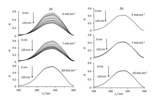
**Figure 4.** Absorbance spectra of RNO ( $2 \times 10^{-5}$  M) in phosphate buffer (pH=7.4) obtained at 5 min intervals during galvanostatic electrolyses with Ti/IrO<sub>2</sub>-SnO<sub>2</sub>-Sb<sub>2</sub>O<sub>5</sub> (a) and Pt (b) anodes. A = 1 cm<sup>2</sup>. T=298 K.
