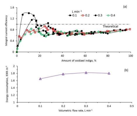
**Figure 7. (a)** Integral current efficiency versus percentage of oxidized indigo in the FM01-LC electrolyzer, evaluated from the electrolyses similar to those from Fig. 5(b). **(b)** Energy consumption versus volumetric flow rate evaluated at 88 % of degradation from the electrolyses similar to those from Fig. 5(b).
