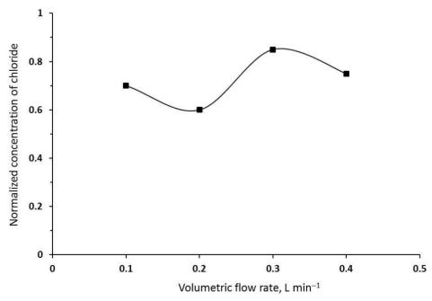
**Figure 6**. Normalized concentration of chloride versus volumetric flow rates evaluated at the end of the electrolyses similar to those from Fig. 5(b). Electrolyte: 1 mM indigo in 0.05 M NaCl. A = 112 cm<sup>2</sup>, j = 7 mA cm<sup>-2</sup>, T = 298 K. Volumetric flow rates are shown in the figure.
