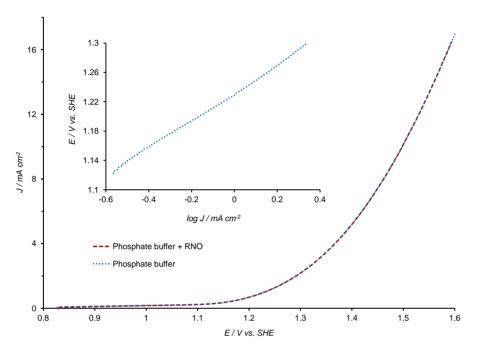
**Figure 3**. Typical linear sweep voltammetries on  $Ti/IrO_2$ - $SnO_2$ - $Sb_2O_5$  anode. Electrolyte: phosphate buffer (pH 7.4), and phosphate buffer +  $2 \times 10^{-5}$  M RNO. The scan rate was 50 mV s<sup>-1</sup>. The inset shows the Tafel plot for J-E curves for phosphate buffer. A = 1 cm<sup>2</sup>. T = 298 K.
