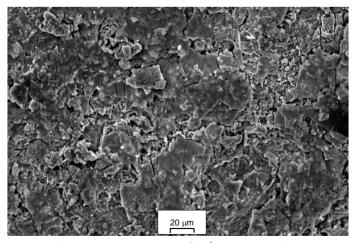
Figure 2. SEM images of Ti/IrO<sub>2</sub>-SnO<sub>2</sub>-Sb<sub>2</sub>O<sub>5</sub>.
