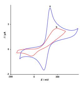
**Figure 4.** CVs of Cu(salophen)/ SPE (a) unmodified SPE (b) in 0.1 M PBS (pH 7.0) containing 100.0  $\mu$ M DA. In all cases the scan rate were 50 mV s<sup>-1</sup>
