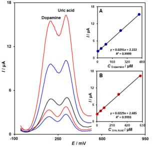
**Fig. 7.** DPVs of Cu(salophen)/SPE in 0.1 M PBS (pH 7.0) containing different concentrations of DA and UA from inner to outer: 5.0 + 5.0, 40.0 + 50.0, 90.0 + 100.0, 250.0 + 300.0 and  $450.0 + 600.0 \mu$ M respectively. Insets (A) plot of  $I_p$  vs. DA concentration and (B) plot of  $I_p$  vs. UA concentrations.
