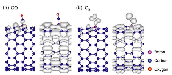
**Figure 4.** Iso-surfaces of squared scattering wave functions of B-doped (14,0) CNT with (a) CO molecule and (b)  $O_2$  molecule at the Fermi energy
