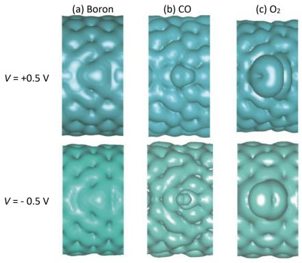
Figure 2. Scanning tunneling microscopy of B-doped (14,0) CNTs: (a) without any adsorbates; (b) with CO molecule; (c) with O₂ molecule. STM images are generated at bias voltages of +0.5 V (upper panel) and -0.5 V (lower panel)
