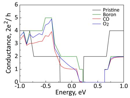
**Figure 3.** Quantum conductance of pristine (14,0) CNT and B-doped (14,0) CNT without any adsorbates, and with CO and O<sub>2</sub> molecules
