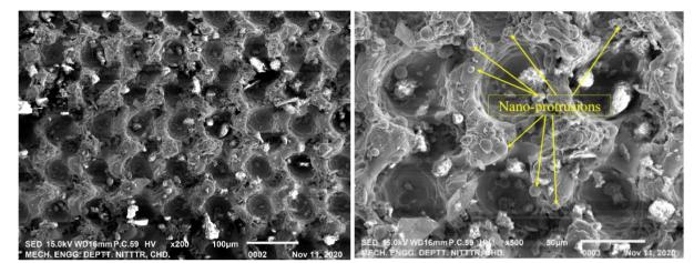
187 *Figure 4.* SEM images of a textured surface with a p/d ratio of 0.7 at different magnification levels
