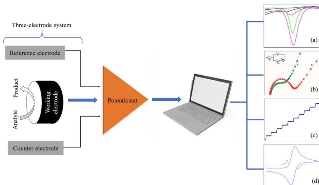
**Figure 5.** Typical electrochemical measurement setup with three electrodes, a working electrode, a reference electrode, and a counter electrode for (a) square wave anodic strip voltammetry (SWASV), (b) electrochemical impedance spectroscopy (EIS), (c) amperometric, and (d) cyclic voltammetry (CV)
