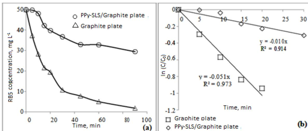
**Figure 5.** Time course profile (a) and first order kinetic profile (b) of RB5 decolourization using Graphite and PPy-SLS-G anodes (Sample 250 mL, Cell : Undivided, RB5 concentration mg L<sup>-1</sup>, Anode: Graphite plate or PPy-SLS/G plate, Cathode : SS plate, Electrolyte: NaCl, Electrode gap : 1 cm)
