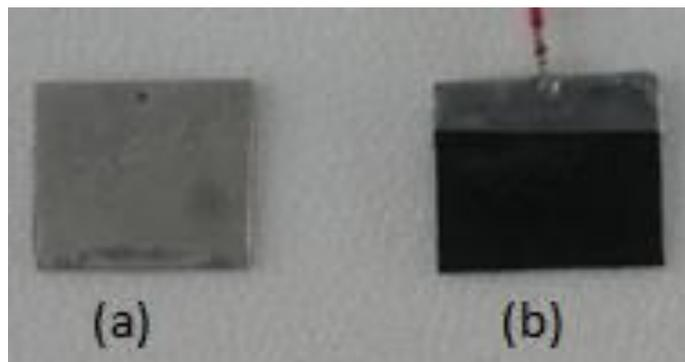
**Figure 2.** Ti (a) and PPy-SLS-Ti (b) plates
