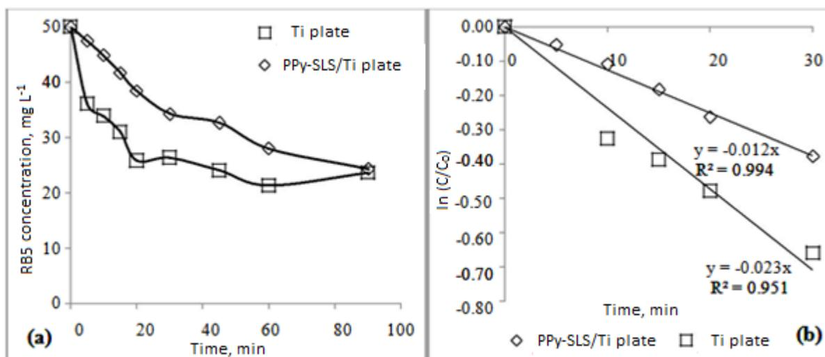
Figure 4. Time course profile (a) and first order kinetic profile (b) of RB5 decolourization using Ti and PPY-SLS-Ti anodes (Sample 250 mL, Cell : Undivided, RB5 concentration mg L<sup>-1</sup>, Anode: Ti plate or PPY-SLS/Ti plate, Cathode : SS plate, Electrolyte: NaCl, Electrode gap : 1 cm)
