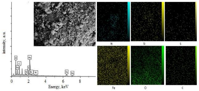
**Figure 6.** EDS spectrum of  $\gamma$ -Fe<sub>2</sub>O<sub>3</sub>@SiO<sub>2</sub>-2-(2-benzothiazolyl azo)-4-methoxyaniline and mapping of Fe, Si, S, N, O, C
