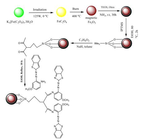
**Scheme 2.** Steps during preparation of  $\gamma$ -Fe<sub>2</sub>O<sub>3</sub>@SiO<sub>2</sub>-2-(2-benzothiazolyl azo)-4-methoxyaniline
