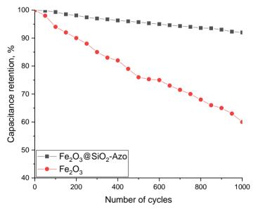
Figure 9. Cycling stability of  $\gamma$ -Fe<sub>2</sub>O<sub>3</sub> and  $\gamma$ -Fe<sub>2</sub>O<sub>3</sub>@SiO<sub>2</sub> -azo ligand electrodes
