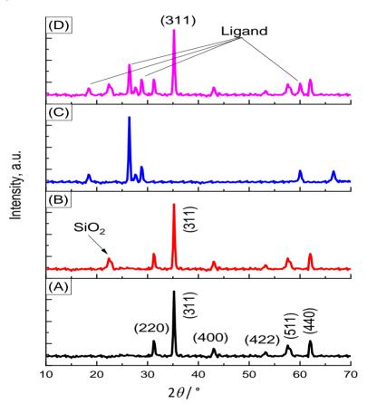
**Figure 3.** XRD patterns of: (A) γ-Fe<sub>2</sub>O<sub>3</sub>, (B) γ-Fe<sub>2</sub>O<sub>3</sub>@SiO<sub>2</sub>, (C) azo ligand, and (D) γ-Fe<sub>2</sub>O<sub>3</sub>@SiO<sub>2</sub>-azo ligand
