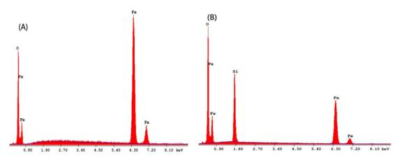
Figure 7. EDX spectra of: (A)  $\gamma$ -Fe<sub>2</sub>O<sub>3</sub> and (B)  $\gamma$ -Fe<sub>2</sub>O<sub>3</sub>@SiO<sub>2</sub>
