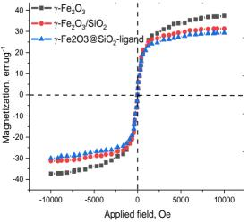
Figure 2. VSM of prepared electrode materials
