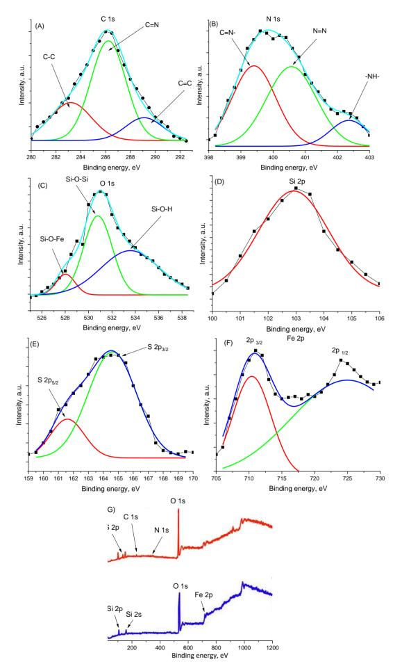
**Figure 4.** XPS of: (A) C 1s, (B) N 1s, (C) O 1s, (D) Si 2p, (E) S 2p, (F) Fe 2p,  $\gamma$ -Fe<sub>2</sub>O<sub>3</sub>@SiO<sub>2</sub>-azo dye and (G) survey spectra of  $\gamma$ -Fe<sub>2</sub>O<sub>3</sub>@SiO<sub>2</sub> and  $\gamma$ -Fe<sub>2</sub>O<sub>3</sub>@SiO<sub>2</sub>-2-(2-benzothiazolyl azo)-4-methoxyaniline
