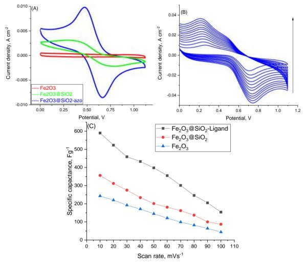
**Figure 8.** CVs of (A)  $\gamma$ -Fe<sub>2</sub>O<sub>3</sub>,  $\gamma$ -Fe<sub>2</sub>O<sub>3</sub>@SiO<sub>2</sub> and  $\gamma$ -Fe<sub>2</sub>O<sub>3</sub>@SiO<sub>2</sub> azo ligand electrodes at 10 mV s<sup>-1</sup>, and (B)  $\gamma$ -Fe<sub>2</sub>O<sub>3</sub>@SiO<sub>2</sub>-azo ligand electrode at different scan rates (10-100 mV s<sup>-1</sup>), (C) specific capacitance of three electrodes at different scan rates
