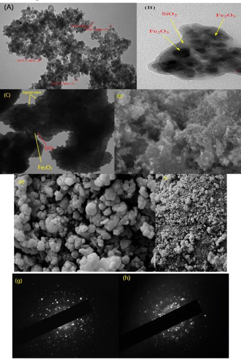
**Figure 5.** TEM images of (A) γ-Fe<sub>2</sub>O<sub>3</sub>, (B) γ-Fe<sub>2</sub>O<sub>3</sub>@SiO<sub>2</sub>, (C)γ-Fe<sub>2</sub>O<sub>3</sub>@SiO<sub>2</sub>-azo ligand; FESEM images of (D)γ-Fe<sub>2</sub>O<sub>3</sub>, (e) γ-Fe<sub>2</sub>O<sub>3</sub>@SiO<sub>2</sub>, (f)γ-Fe<sub>2</sub>O<sub>3</sub>@SiO<sub>2</sub>-azo ligand, and SAED images of: (g) γ-Fe<sub>2</sub>O<sub>3</sub>, (h)γ-Fe<sub>2</sub>O<sub>3</sub>@SiO<sub>2</sub>-azo ligand
