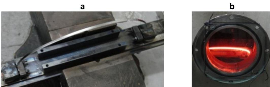
**Figure 3.** (a) Filaments made out of the heat shields (b) Hot filament as viewed by the pyrometer
