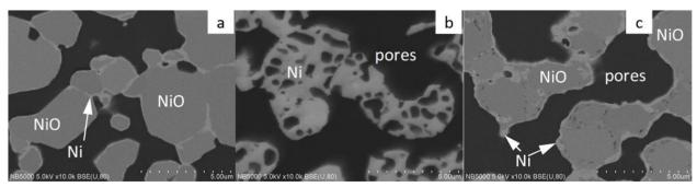
**Figure 3.** SEM images of NiO sample after (a) reduction in mixture 5 %  $H_2$ -Ar at 600 °C; (b) reduction in pure  $H_2$  at 600 °C; (c) RedOx in mixture 5 vol. %  $H_2$ -Ar at 600 °C
