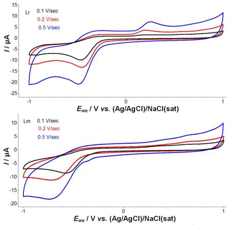
**Figure 7.** CVs recorded of the Lr and Lm in the presence of 0.25 mg mL $^{-1}$  of lipase at different scan rate, E / V vs. Ag/AgCl
