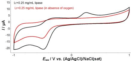
**Figure 6.** CVs recorded of Lr in 0.1 M KNO<sub>3</sub> and in the presence of 0.25 mg mL<sup>-1</sup> lipase with and without oxygen; E / V vs. Ag/AgCl, 0.5 V s<sup>-1</sup>
