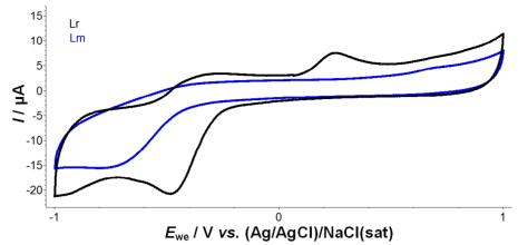
**Figure 8.** CVs recorded of the Lr and Lm in the presence of 0.50 mg mL<sup>-1</sup> of lipase; E/V vs. Ag/AgCl, 0.5 V mV  $s^{-1}$
