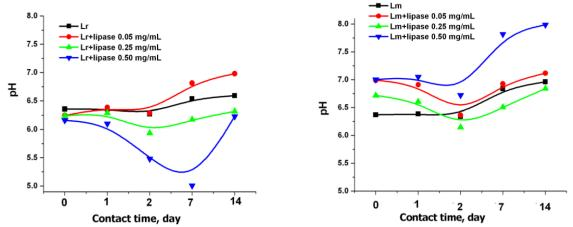
**Figure 1.** Time evolution of pH of the solutions containing the rigid and mobile ligand (Lr and Lm) with and without lipase
