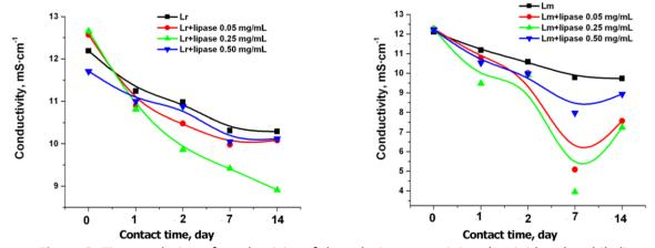
**Figure 2.** Time evolution of conductivity of the solutions containing the rigid and mobile ligand (Lr and Lm) with and without lipase
