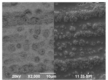
**Figure 4.** Scanning – electron image of the pink-lilac coatings with content 64.9 wt. % Sb, 35.1 wt. % Cu and thickness 3.6 μm.
