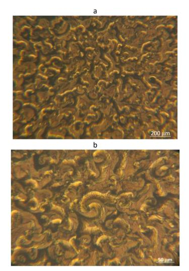
**Figure 6.** Optical images of the coating at different magnifications with spatio-temporal structures, obtained at:  $j = 0.4 \text{ A m}^{-2}$ , deposition time- 240 min, thickness -23.76  $\mu$ m
