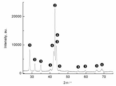
**Figure 7.** X-Ray diffractogram of the sample, shown in Figure 6. The registered phases are marked with numbers: 1 - Sb;  $2 - Cu_{2.6}Zn_{1.4}$ ;  $3 - Cu_2Sb_1$ ;  $4 - Cu_{11}Sb_3$ .
