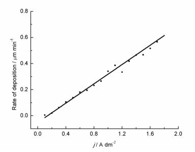
**Figure 3.** Effect of the current density on the deposition rate of the Cu-Sb coatings. The composition of the electrolyte is presented in Table 1.
