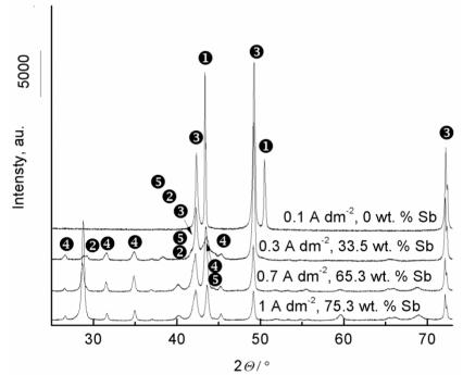
**Figure 5.** X-ray diffractograms of Cu-Sb coatings with different antimony content, obtained in the electrolyte, presented in Table 1. The existed phases are marked with numbers  $1 - Cu; 2 - Sb; 3 - Cu_{2.6}Zn_{1.4}; 4 - Cu_2Sb_1; 5 - Cu_{11}Sb_3$
