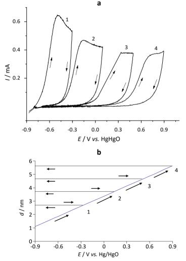
**Fig. 3.** (a) Multiple cycle sequences at increasing final anodic voltage of Nb recorded in 1M KOH; 1, 2, 3, and 4 represent number of cycle, (b) Simulated film thickness growth in each subsequent cycle
