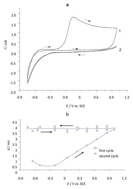
**Fig. 2.** (a) Voltammograms of Nb recorded in 10 M H<sub>2</sub>SO<sub>4</sub>, 1 – first cycle, 2 – second cycle; (b) Simultaneous determination the thickness of passive film by ellipsometry
