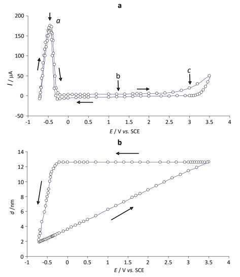
**Fig. 1.** (a) Potentiostatic I – E curve obtained on electropolished Ti surface in 3 M H<sub>2</sub>SO<sub>4</sub>, (b) Simultaneous determination the thickness of passive film by ellipsometry
