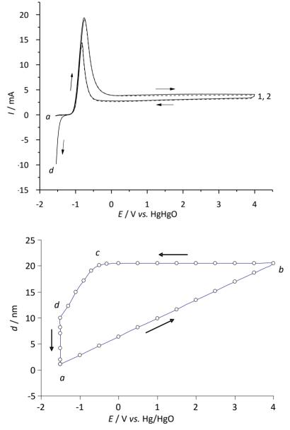
Fig. 4. (a) Voltammograms of Nb recorded in 6 M KOH, a – initial current at potential of -1.5 V, d – final current at potential of -1.5 V, 1 – first cycle, 2 – second cycle;
