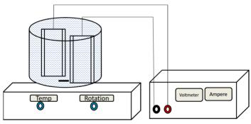
Figure 2. Laboratory scale electrocoagulation cell
