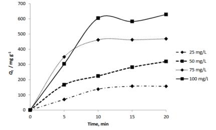
**Figure 6.** Effect of initial concentration on the electrocoagulation removal of ARS  $(T = 30 \ ^{\circ}C, \ pH = 7, \ j = 21.5 \ A \ m^{-2} \ [NaCl] = 2 \ g \ L^{-1})$
