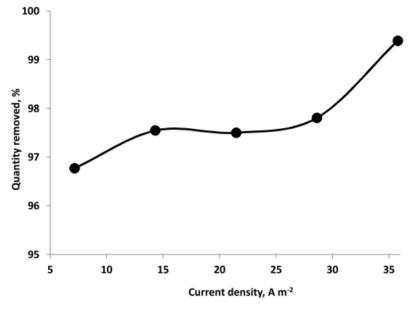
**Figure 3.** Effect of current density on colour removal  $([ARS] = 50 \text{ mg L}^{-1}, T = 30 \,^{\circ}C, pH 7.0 \text{ and } [NaCl] = 2 \text{ g L}^{-1}).$
