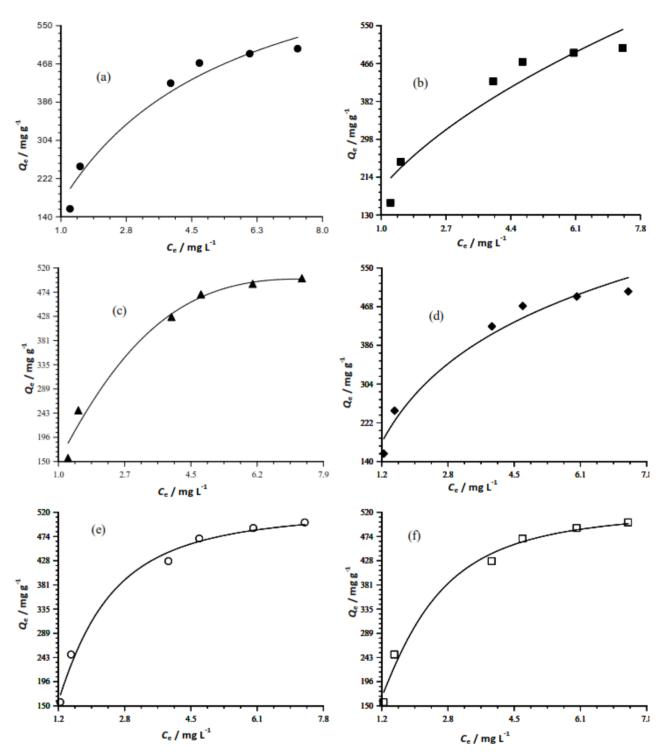
*Figure 7.* Least square plots of the (a) Langmuir, (b) Freundlich, (c) Redlich–Peterson, (d) Temkin (e) Dubinin–Radushkevich and (f) Sips isotherms for electrocoagulation of Alizarin S dye at 30 °C.
