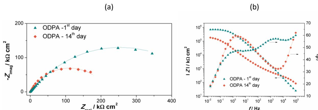
**Figure 7.** Nyquist (a) and Bode (b) impedance spectra for ODPA treated samples for the 1<sup>st</sup> and 14<sup>th</sup> day of immersion in 3 % NaCl solution.
