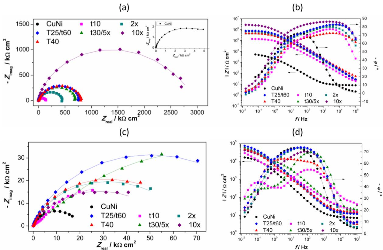
Figure 4. EIS – Nyquist and Bode plots: (a) and (b) after one hour, and (c) and (d) 14<sup>th</sup> day of exposure to 3% NaCl. Symbols - experimental data; solid lines - modelled data according to electrical equivalent circuits given in Fig. 5
