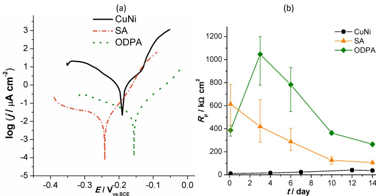
**Figure 6.** Comparison of equally prepared SA and ODPA films – results of polarization measurements: (a) polarization curves recorded after one hour immersion in 3 % NaCl, and (b) polarization resistance as a function of immersion time for blank and treated samples.
