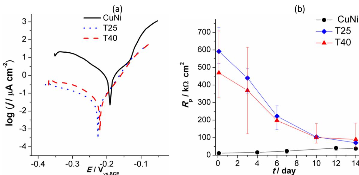
**Figure 1.** Influence of temperature between spraying: (a) polarization curves recorded after one-hour immersion in 3 % NaCl and (b) polarization resistance as a function of immersion time for blank and treated samples
