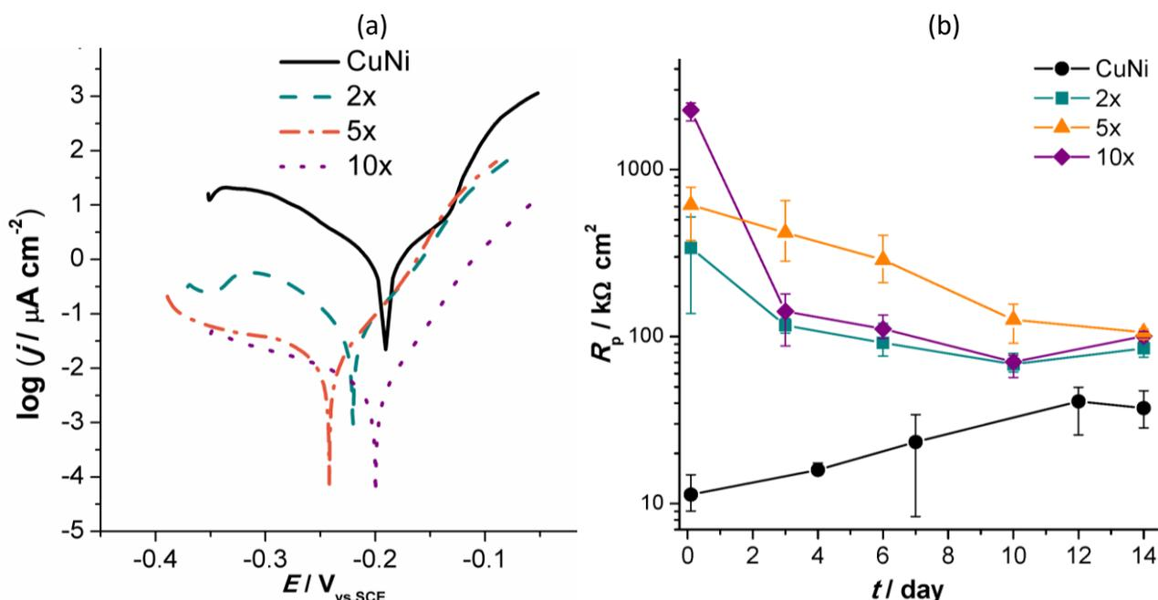
**Figure 3.** Influence of the number of spraying – results of polarization measurements: (a) polarization curves recorded after one hour of immersion in 3 % NaCl, and (b) polarization resistances as a function of immersion time for blank and treated samples
