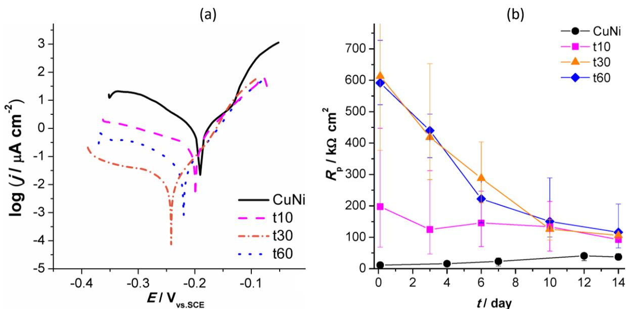
**Figure 2.** Influence of time between spraying – results of polarization measurements: (a) polarization curves recorded after one hour immersion in 3 % NaCl, and (b) polarization resistance as a function of immersion time for blank and treated samples.
