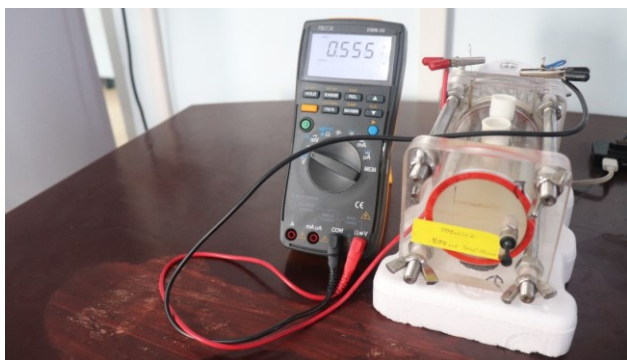
Figure 2. Batch operation on a single chamber microbial fuel cell (SCMFC)
