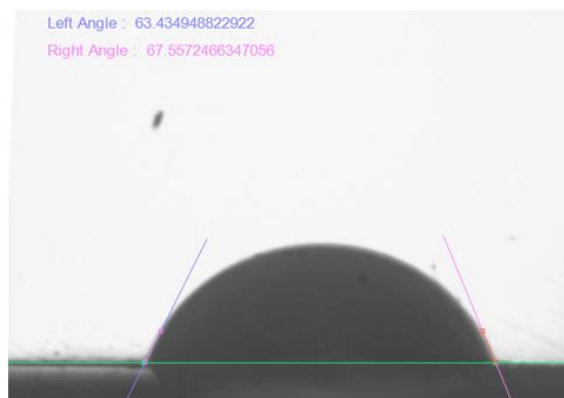
Figure 4. Wetability test of IL-MoO 3
