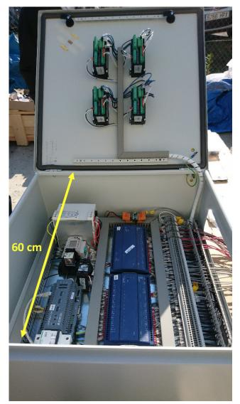
FIG. 5 First BEMS of prototype for the control of the LHTES and SHMRU (assembly by CARTIF). Image by D'Appolonia.
