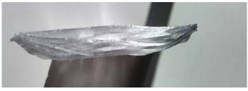
FIG. 3 Cross section of the panels, showing the elongated cells in the insulation core and the channels in the external water layer.
