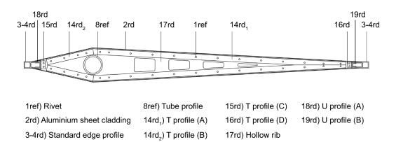
FIG. 14 Redesigned sunscreen panel cross section detail, alternative 1
