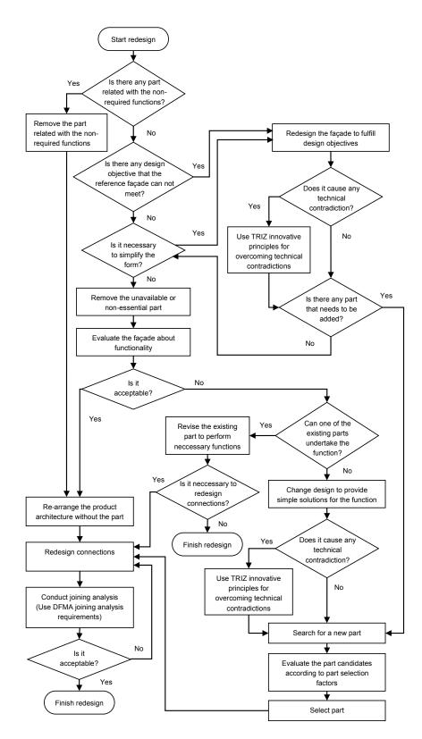
FIG. 9 Phase IV: Redesign of the reference façade, process flowchart
