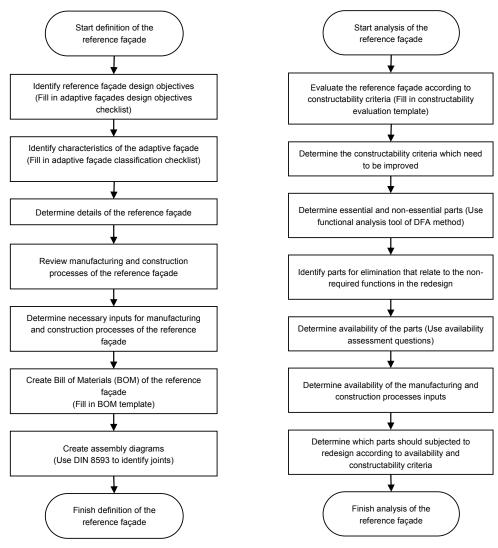
FIG. 7 Phase II: Definition of reference façade, process flowchart
