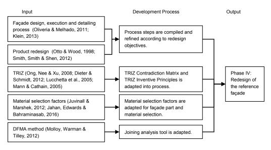
FIG. 5 Phase IV: Redesign of the reference façade, development of process steps
