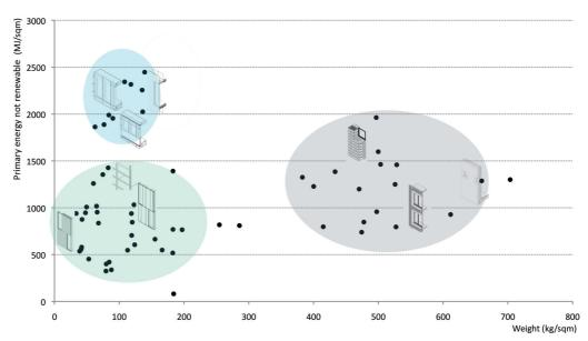
FIG. 1 Embodied energy in different façade typologies. (blue: double façades; green: post-and-beam construction; grey: solid façades) (Hildebrand, 2014)
