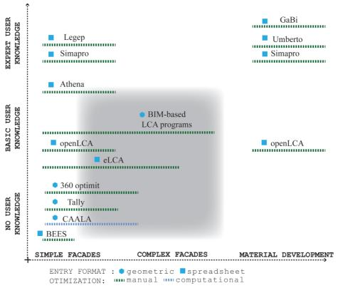
FIG. 12 LCA Software products organised according to user knowledge and planning assignment. The grey field marks the most suitable products for facade design and engineering.
