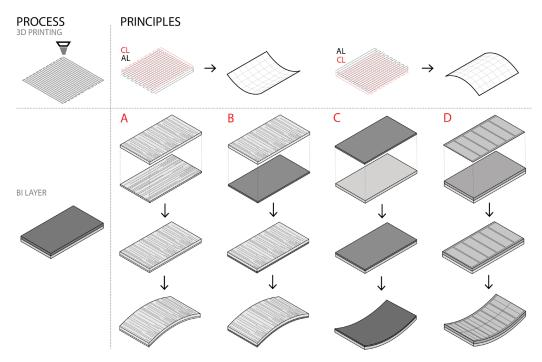
FIG. 4 Manufacturing principles
