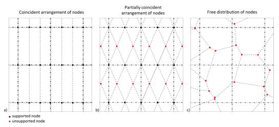
FIG. 4 The relationship between façade grids and axial controlling lines of the structure: a) coincident arrangement, b) partially coincident arrangement, c) free distribution of nodes
