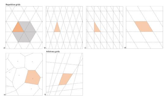
FIG. 5 Representation of a simplified typology based on the number of sides of the polygon: a) triangular (hexagonal grid); b) isosceles triangle grid; c) right triangle grid; d) quadrilateral grids; f) Voronoi tessellation; e) arbitrary grid
