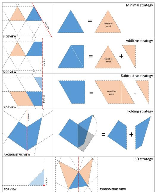
FIG. 7 Different edge panel strategies. From top to bottom: minimal, additive, subtractive, folding, and 3D
