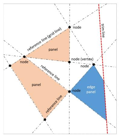
FIG. 1 Diagrammatic presentation of the basic definitions used in the paper (description provided in the diagram)
