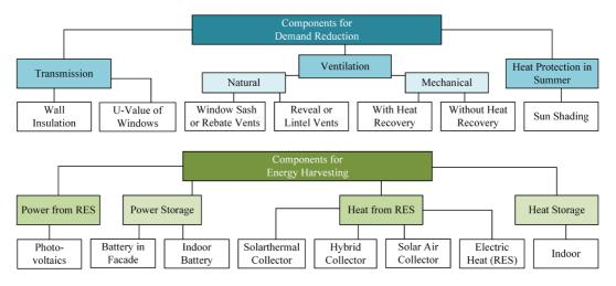
FIG. 6 Components for demand reduction and energy harvesting
