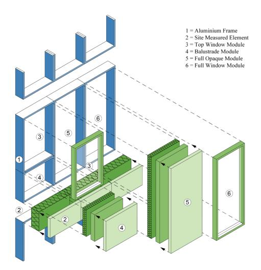
FIG. 5 Main elements of the PLUG-N-HARVEST system
