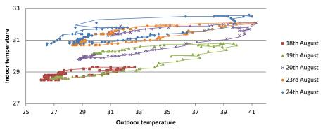
FIG. 9 Indoor and outdoor temperature of the first floor room with shading device (18th - 24th August)
