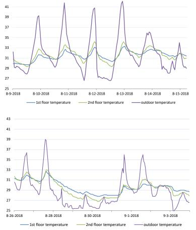
FIG. 10 Outdoor and indoor temperature of the two floors (°C) [above] 9th - 15th August (unshaded façade)[below] 26th August - 3rd September (aluminium shading devices)
