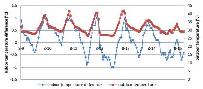
FIG. 15 The indoor temperature difference of the two floors (both bare façade) and outdoor temperature (09th until 15th of August)
