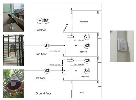
FIG. 4 Locations of the measurement equipment
