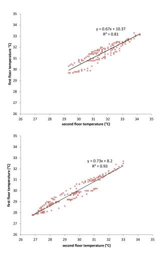
FIG. 11 Scatter plot of indoor temperature of the two floors (°C) [above] 9th - 15th August (unshaded façade)[below] 26th August - 3td September (aluminium shading devices)
