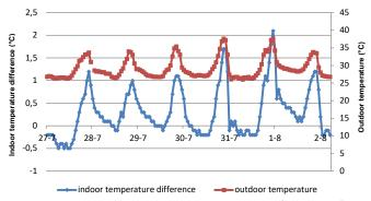
FIG. 14 The indoor temperature difference between first floor (green façade) and second floor (bare) and outdoor temperature (July  $27^{th}$  - August  $2^{nd}$ )
