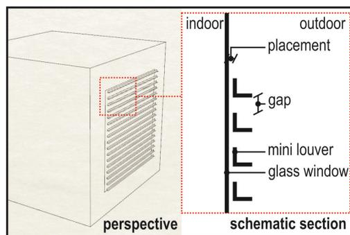
FIG. 7 Schematic of horizontal *koshi* mini-louvres design
