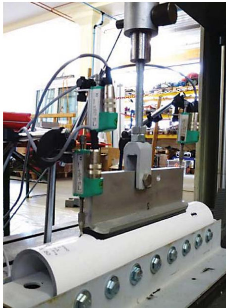
Figs. 9, 10. Test: gluing the pull holder and according FE model (Images: Michel).
