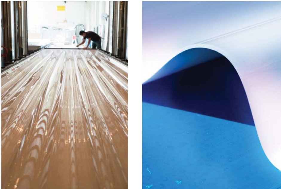
Figs. 5, 6. Deep drawn panel in the oven – Wave section made of co-extruded acrylic glass (Images: Michel).
