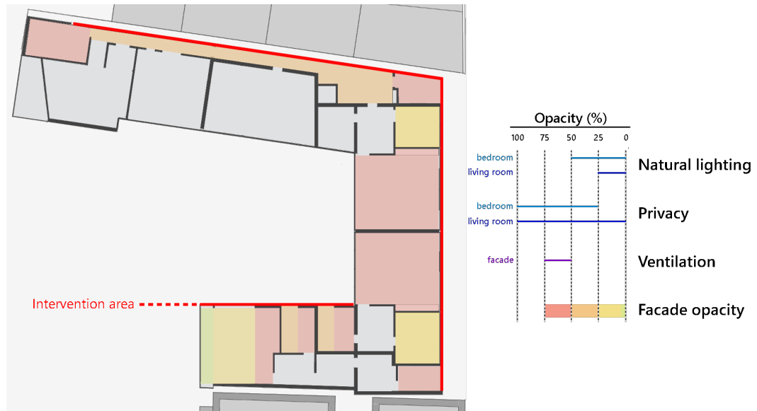
FIG. 7 Case study plan: the red lines represent the façade intervention areas and the coloured areas the different opacity levels explained in the right-side diagram.
