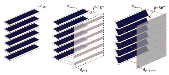
FIG. 6 Different areas that can be used as reference area  $A_{ref}$  to calculate the solar thermal efficiency  $\eta$ . Left: Overall slat absorber area  $A_{abst.t} \approx 2.67 m^2$ . Centre: Projected slat area  $A_{proj}$  for exemplary slat tilt angle of  $\beta = 10^{\circ}$ . Right: Maximum projected slat area  $A_{proj}$  for scale tilt angles of  $\beta \geq 56^{\circ}$ .
