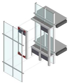
FIG. 8 STVB installation in Scenario 1 on a multi-storey ventilated double-skin façade
