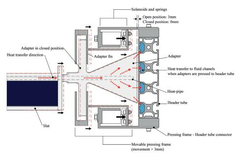
FIG. 4 Schematic horizontal cross-section of the switchable thermal coupling mechanism used as heat transfer component in the STVB test sample. Red arrows indicate the heat flow from slat through heat pipe and adapter to the fluid in the header tube. Black arrows indicate the movement of the switchable thermal coupling mechanism from open to closed position. The dashed red lines indicate the position of slat, adapter, and movable pressing frame when the switchable thermal coupling is closed.
