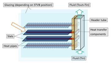
FIG. 1 Main components of a solar thermal venetian blind positioned between an outer and an inner glazing pane. The increase between fluid inlet temperature  $T_{in}$  and fluid outlet temperature  $T_{out}$  illustrates the harvesting of solar thermal heat. The blind mechanism for retracting and tilting the slats is not shown.
