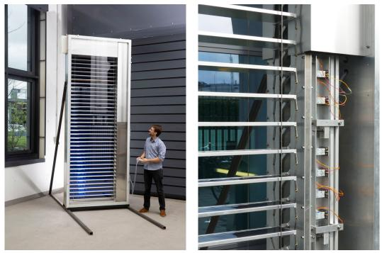
FIG. 5 Left: Test sample of double skin façade element ( $1.4 \text{ m} \times 3.6 \text{ m}$ ) with integrated solar thermal venetian blind seen from the exterior side. Right: Switchable thermal coupling mechanism with springs and solenoids mounted in the test sample, upper part covered with cover sheets.
