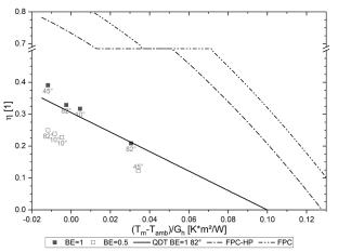
FIG. 7 Efficiency curves  $\eta$  of STVB test sample for  $T_{ini} \approx T_{amb}$  as function of mean fluid temperature  $T_{m}$ , ambient temperature  $T_{amb}$ , and hemispherical irradiance  $G_b$  compared to reference collectors (cf. TABLE 3). Slat tilt angles  $\beta$  noted as label for each data point. Reference area  $A_{abstotal} = 2.67 \text{ m}^2$  used for the STVB.
