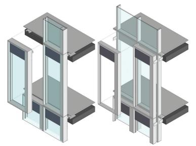
FIG. 9 STVB installation in Scenario 2 as part of double skin unitised façade (left); as an additional stand-alone element on an existing unitised or stick façade system (right)
