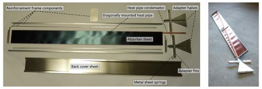
FIG. 3 Left: Slat components. Right: Back surface of a slat with diagonally mounted heat pipe and triangular adapter in the foreground (back cover sheet removed).
