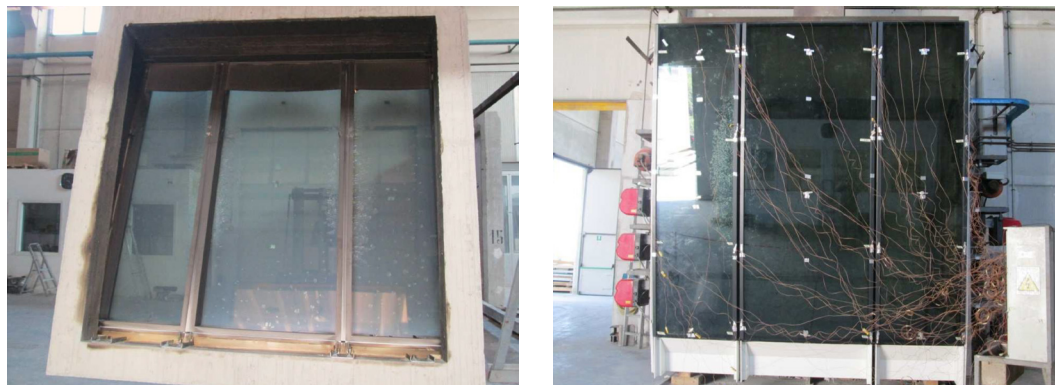
FIG. 25 Façade mock-up after the laboratory test (on the left). Façade mock-up with thermocouples test equipment (on the right)
