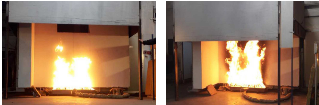
FIG. 2 Images of laboratory tests to evaluate the fire behaviour of an opaque façade solution: ignition phase (left) and steady phase after 10 minutes (right)
