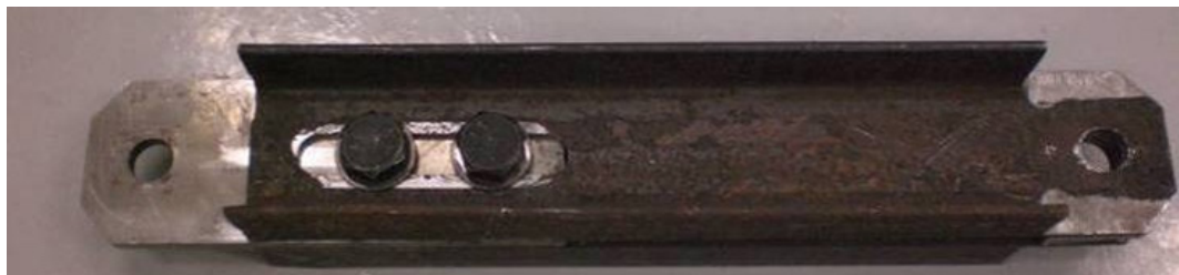
FIG. 4 Linear-motion friction damper (Chan & Hu, 2016)
