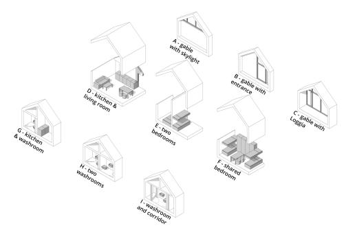
FIG. 1 Module typologies for different types of emergency accommodation depending on number of persons, duration of stay, and level of comfort
