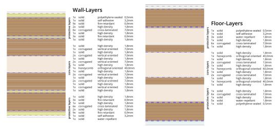
FIG. 5 Layer structure of the wall and floor segments
