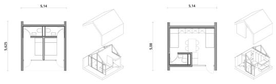
FIG. 2 [left] temporary shelter, [right] emergency shelter
