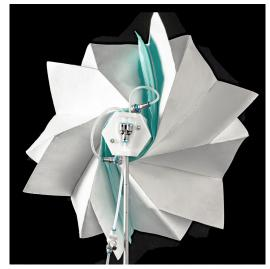
FIG. 9 Additively joined pneumatic actuators. Copyright by ILEK
