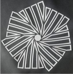
FIG. 6 3D-printed skeletal polymer structure on polyester fabric. Copyright by ILEK
