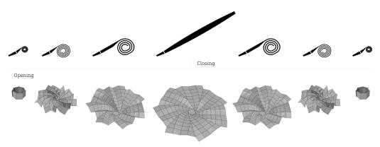
FIG. 8 Opening and closing mechanism. Copyright by ILEK
