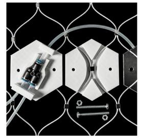
FIG. 10 Connection joint for PAOSS elements. Copyright by ILEK
