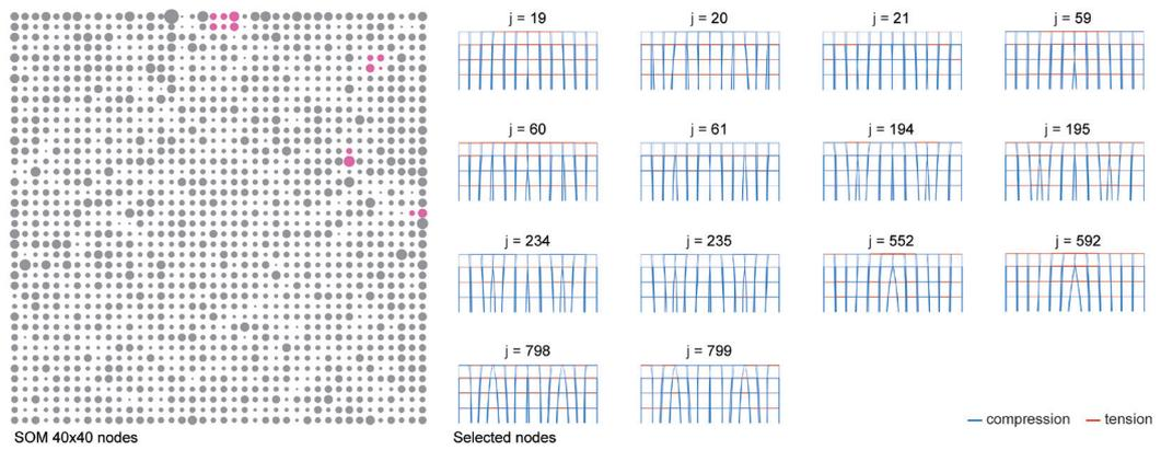
FIG. 9 Selection procedure for Option A ( $j = 61$ ;  $k = 16'562$ ). Representative design options (right) for the 14 nodes retained from the  $40 \times 40$  SOM (left) after the application of hard filters on the total mass  $\text{totMass}$  (5<sup>th</sup> percentile) and the mean value of daylight factor  $\text{DF\_mean}$  (90<sup>th</sup> percentile).
