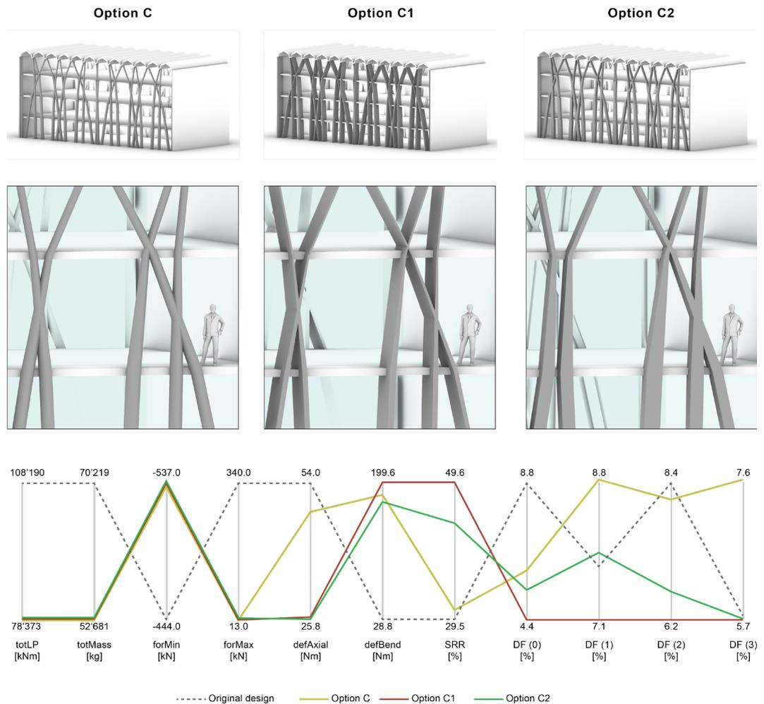
FIG. 11 Three different materialisations of the same form diagram. While keeping constant values for the cross-section areas, rectangular cross-sections with different proportions (Option C1 and C2) are compared to the circular hollow sections of Option C.
