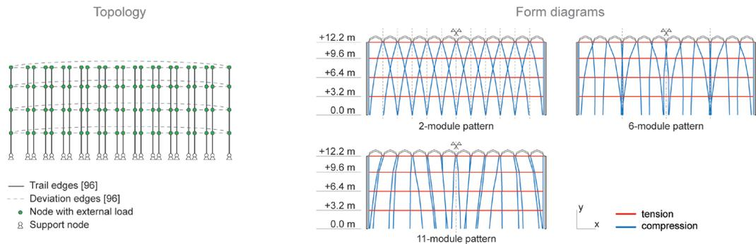
FIG. 5 Generation of various form diagrams (right) via the CEM. The topology (left), the floor heights and the load-case are kept constant, and only the distribution of deviation force magnitudes (*devMag*) is varied
