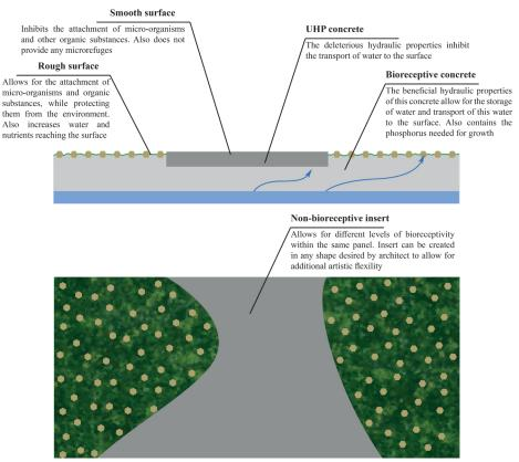
FIG. 2 Overview of the final panel design
