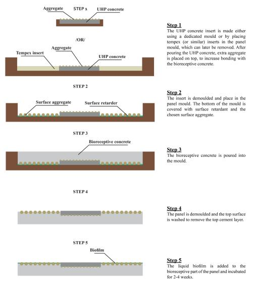
FIG. 3 Graphical overview of the panel production process
