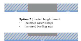
FIG. 1 Sectional overview of different insert options
