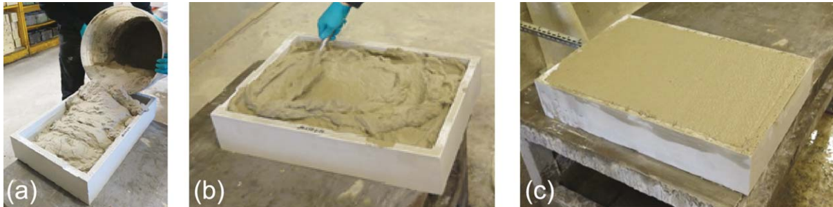
Fig. 9. Manufacturing of UHPC-CLC small-scale samples. (a) Cast of CLC. (b), (c) Homogenous distribution of CLC in the UHPC box.
