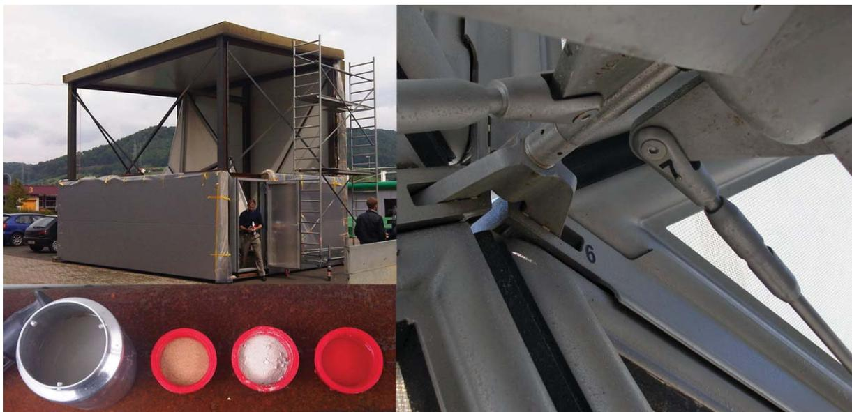
**Fig. 24.** Sand, dust, and seawater was brought from Abu Dhabi and sprayed on full-scale components during life cycle tests. Inside a controlled testing chamber the dynamic unit was monitored over 30,000 cycles. This was the equivalent of eighty years of operation compressed into two months.
