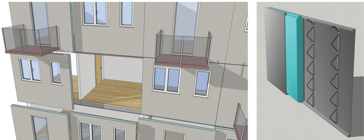
**Fig. 1.** SESBE facade concept (left) and innovative sandwich facade element (right).
