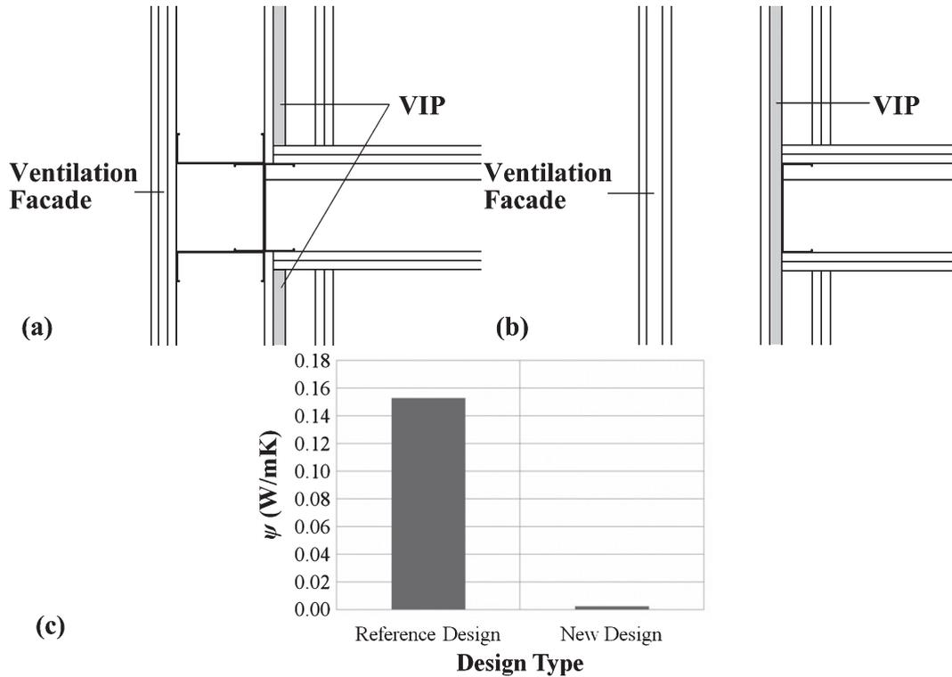
**Fig. 10.** Design modification of the external wall – internal wall junction: a) schematic diagram of the reference junction, b) schematic diagram of the modified junction and b) linear thermal transmittance of the two design solutions.
