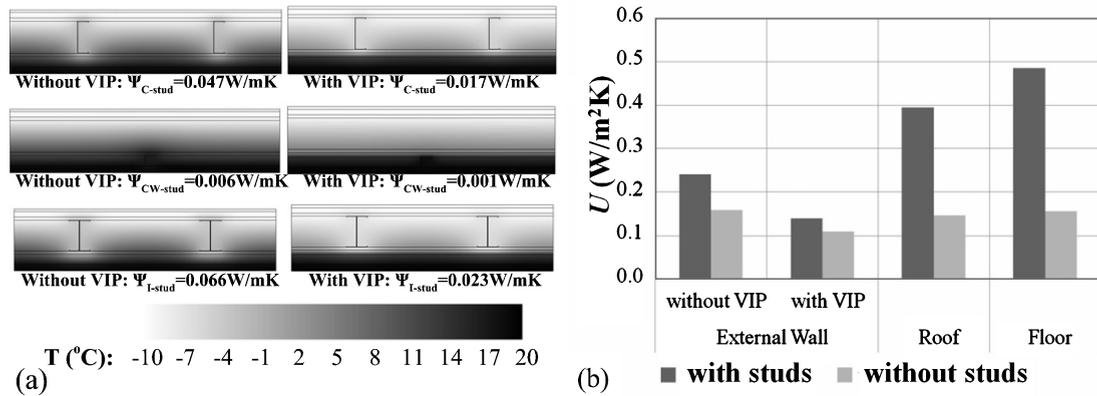
Fig. 3. a) Temperature contours of the external wall for all the types of the studs without and with the VIPs and b) impact of the studs on the U-value for all the building elements.
