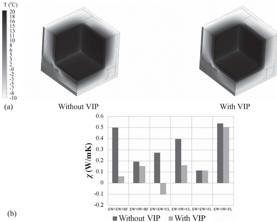
Fig. 5. a) Temperature contours of the external wall – external wall – roof junction without and with the VIPs and b) point thermal transmittance of all 3D junctions without and with the VIPs.
