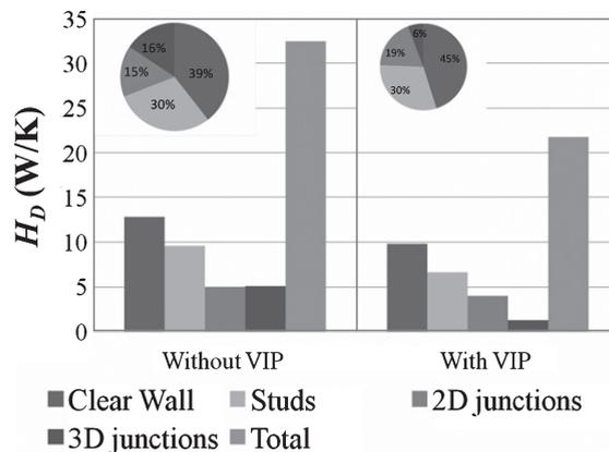
Fig. 6. Impact of thermal bridges on the overall thermal transmittance without and with the VIPs.
