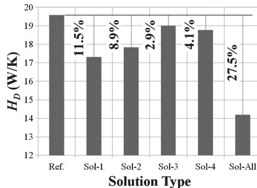
**Fig. 11.** Overall thermal transmittance of the building with different design solutions.
