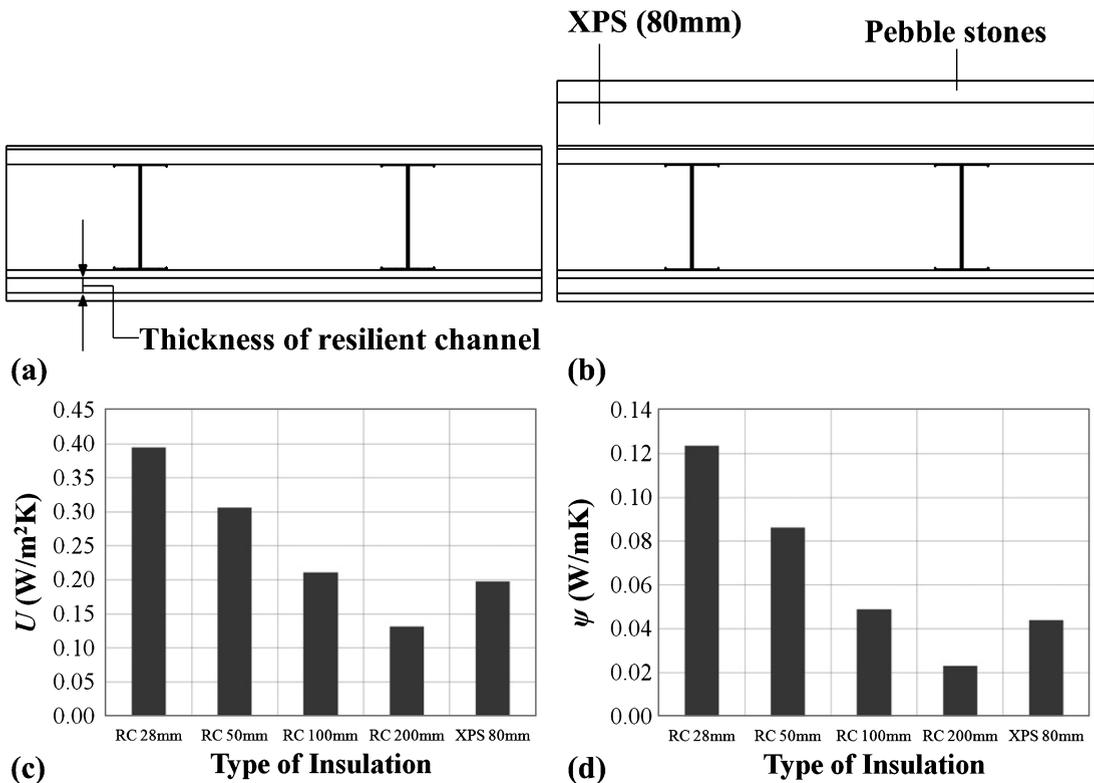
**Fig. 7.** Design modification of the roof configuration: a) schematic diagram of the wall assembly with different thicknesses for the resilient channel, b) schematic diagram of the wall assembly with an XPS layer on the top, c)  $U$ -value of the wall assembly for different types of insulation and d) linear thermal transmittance of the wall assembly's studs for different types of insulation.
