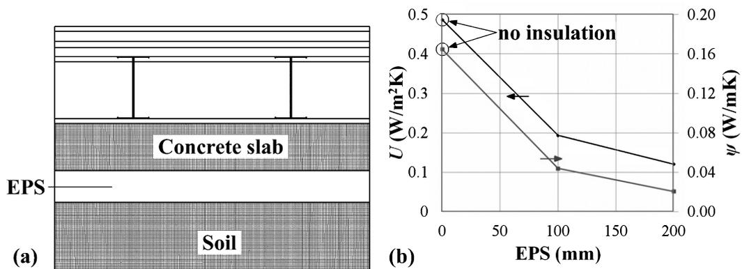
**Fig. 8.** Design modification of the floor configuration: a) schematic diagram of the wall assembly and b)  $U$ -value of the wall assembly and linear thermal transmittance of the wall assembly’s studs for different thickness of EPS between the foundation and the soil.
