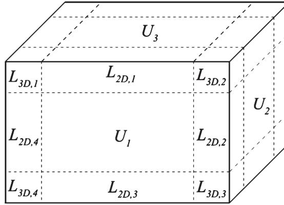
Fig. 2. Partitioning of building into 1D, 2D and 3D geometrical models.
