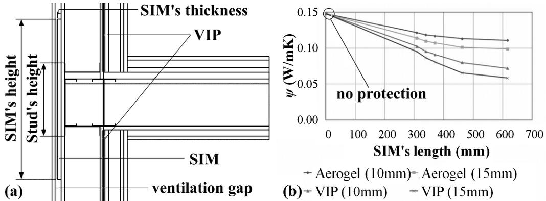
Fig. 9. Design modification of the external wall – ceiling junction: a) schematic diagram of the junction and b) linear thermal transmittance of the junction with different SIM protection.
