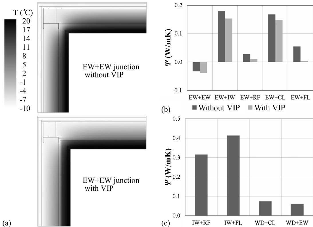
**Fig. 4.** a) Temperature contours of the external wall – external wall junction without and with the VIPs, b) linear thermal transmittance for the 2D junction affected by the VIPs and c) linear thermal transmittance for the 2D junction not affected by the VIPs.
