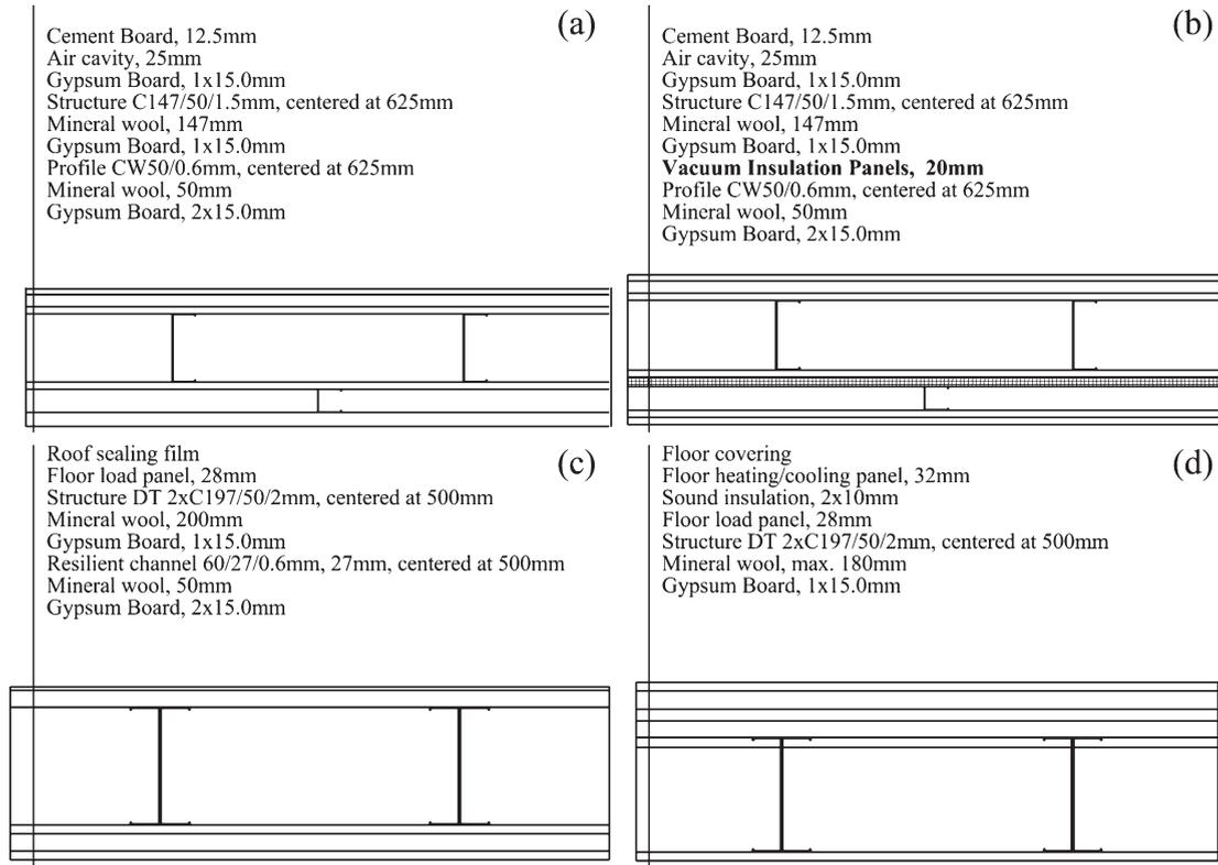
**Fig. 1.** Schematic diagram of the configurations of the building elements: a) External wall without VIP, b) External wall with VIP, c) Roof and d) Floor.
