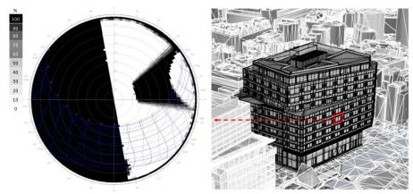
FIG. 6 East Elevation, shading mask and localisation of the assessed bay.
