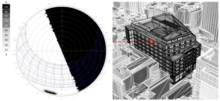
FIG. 4 West Elevation, shading mask and localization of the assessed bay.
