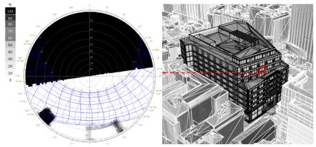
FIG. 5 South Elevation, shading mask and localization of the assessed bay.
