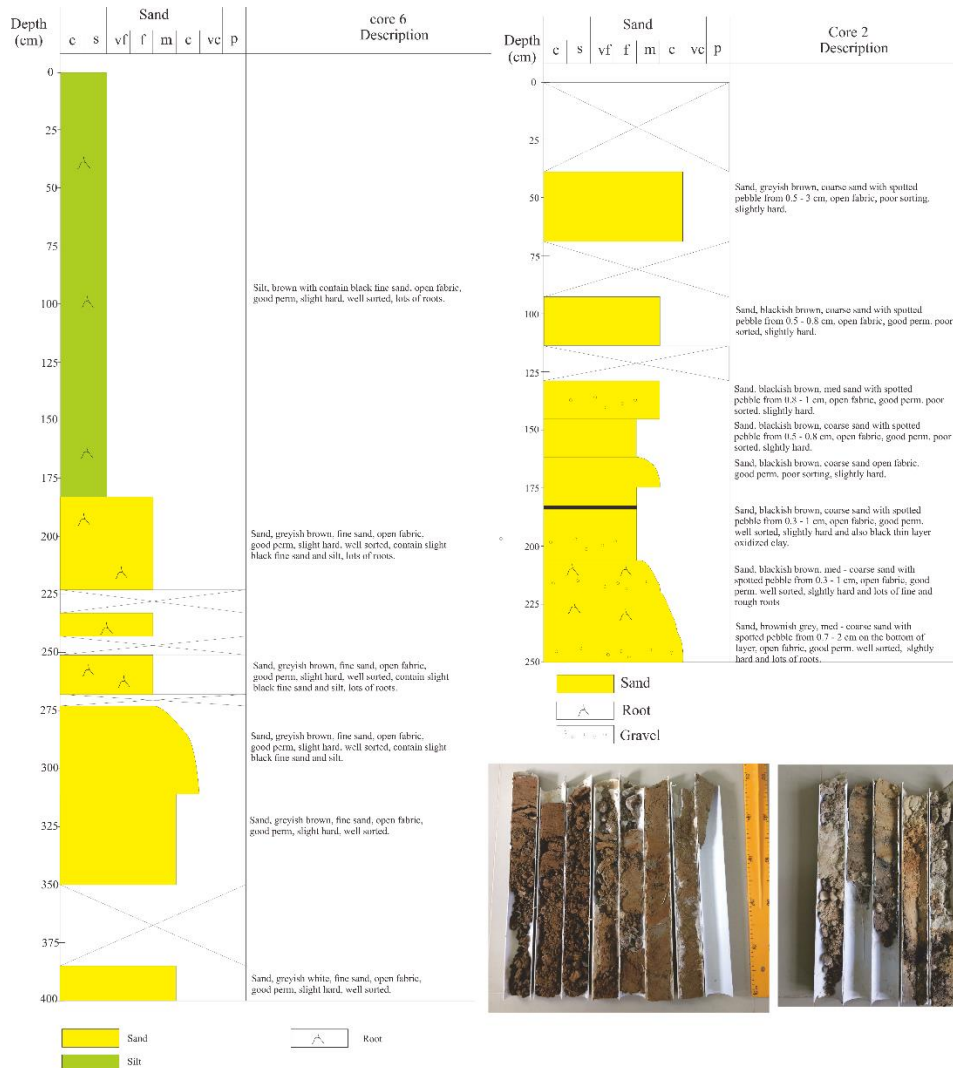
Fig 6. Core sampling and log description of core sampling
