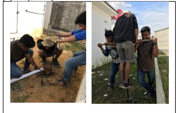
Figure 2. The sampling process using the hand auger method
