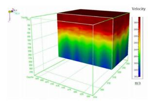
Fig. 3. Interval Velocity Model.
