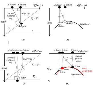
**Fig. 1.** (a) Reflections on the medium with constant lateral velocity, (b) travel time curve from image (a) with the peak just below the geophone (datum B) the recipient, (c) reflection that occurs on the medium with lateral velocity changes, (d) there is an error in the peak position of the travel time that is no longer right under the receiving geophone.
