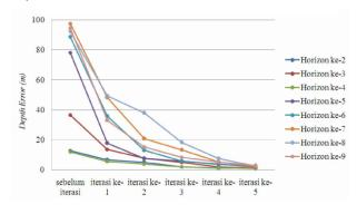
**Fig. 9.** Graph of the relationship between the number of tomographic iterations and the depth error of well 1 and after Tomography (1st-5th iteration)
