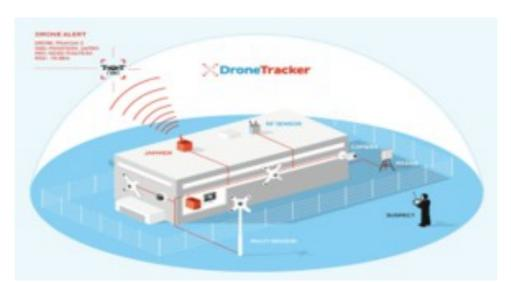
*Note.* A Drone Tracker sensing and detecting a drone in flight in readiness for counter response (Joo-hye, 2019).
