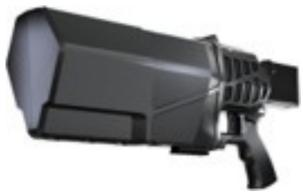
*Note.* An Australian jamming gun for shooting down an invading drone. (Source: https://openworksengineering.com/skywall-patrol/)
