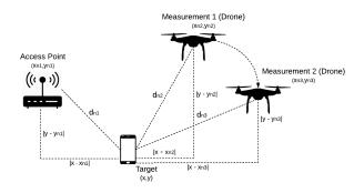
Figure 2. Example of Trilateration with drones
