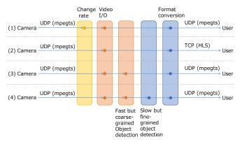
**Figure 2.** Examples of processing in video transfer. (1) Video providers change video frame or bit rates. (2) Video providers distribute video to multiple users. (3) Object detection with only a standard part is executed. (4) Object detection with a new part is executed.
