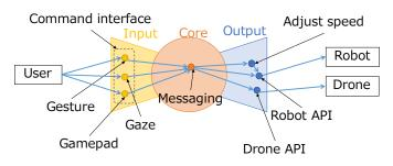
Figure 5. Robot operation based on a core/periphery structure.
