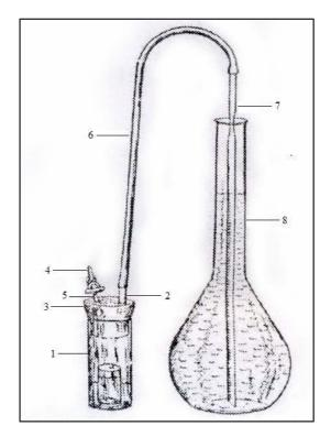
**Figure 2:** The composition of the apparatus Numbers correspond to the above explanation. When the small pipe (No. 7 in the Figure 2) is put inside the bottle, the water level must correspond to the beginning of the gradation of the small pipe.
