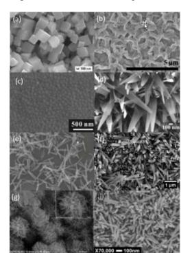
Fig. 1. Nanostructure of  $\alpha$ -Fe<sub>2</sub>O<sub>3</sub>; (a) microcubes, (b) nanowires, (c) nanotube, (d) nanoflakes, (e) nanorods, (f) microstructure orientation, (g) sea-urchin shaped, and (h) worm-shaped
