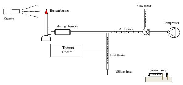
Fig. 1. Laminar burning velocity and flame height test apparatus.
