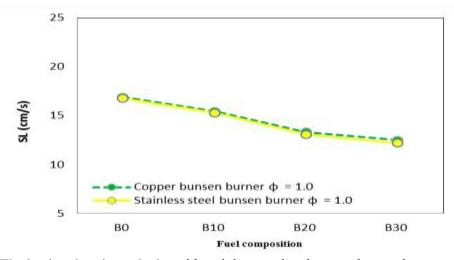
Fig. 5. The laminar burning velocity with stainless steel and copper bunsen burners at  $\varphi = 1.0$
