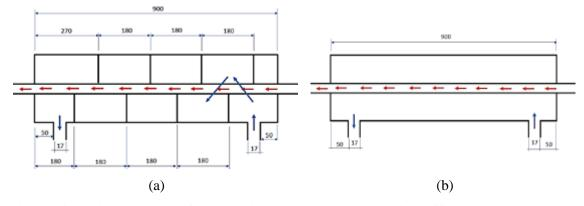
Fig. 3. Dimensions and water flow direction (a) Heat exchanger with baffle, (b) Heat exchanger pipe without baffle
