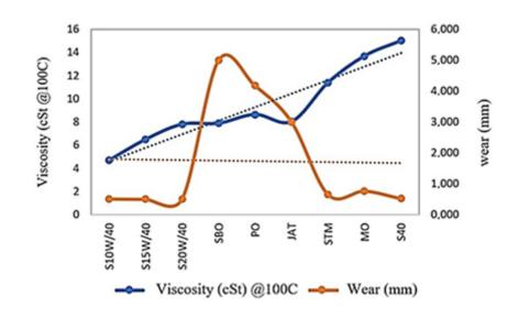
Fig. 3. Graph Viscosity – Wear [16-21]
