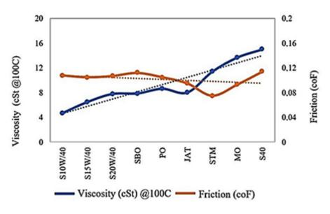
Fig. 2. Graph of Viscosity - Coefficient of friction [16-21]
