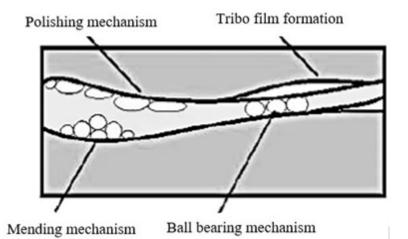
Fig. 1. Lubrication mechanism on two contact surfaces for lubricating nanoparticles [9].
